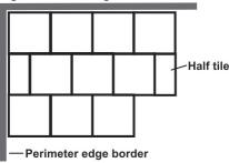
Once installation is complete, install the last two remaining perimeter borders, make sure they are as tight as possible against the tiles.
